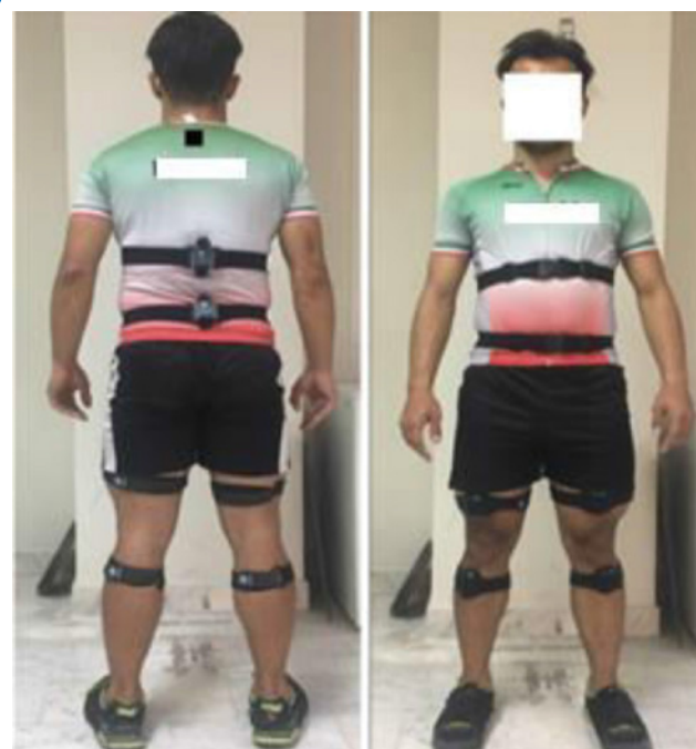
Figure 1. Location of inertial sensors on the subject's body.
