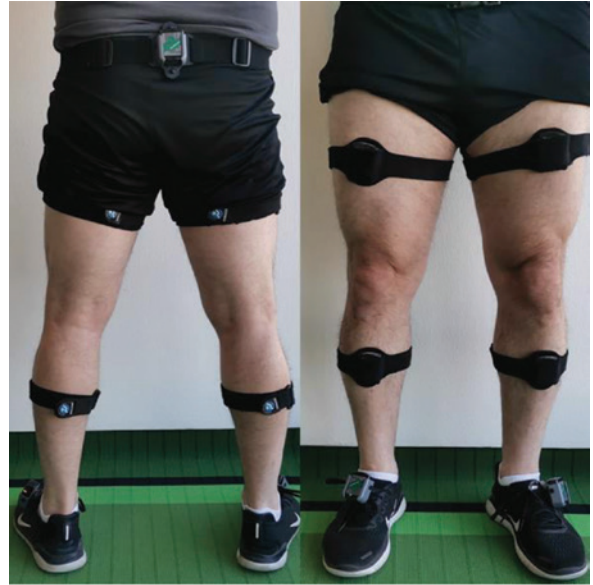
Figure 1. The position of the seven MyoMotion sensors. The pelvic sensor was attached to the bony area of the sacrum. The thigh sensors, they were attached in the frontal side on the lower quadrant of the quadriceps, slightly above the kneecap, and area of lowest.
