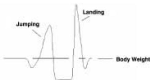
Figure 1. Physiological mechanical stimulation. The Zetos™ bioreactor system is capable of producing dynamic mechanical stimulation in specific waveforms mimicking physiological relevant patterns of exercise. We have used a high impact stimulus using the repetition of the waveform shown above for a jumping signal as obtained from force platform measurements.
