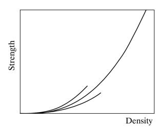
**Figure 6.** Schematic drawing of the power function between apparent density and strength. The thick curve shows the "natural" relationship. The two other curves indicate how treatment regimes might affect the relationship.
