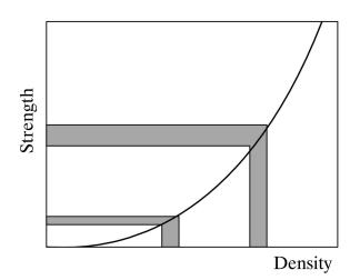
**Figure 7.** Schematic drawing of the power relationship between apparent density and strength. The effect of early and late treatment is indicated. Early treatment (at the steep part of the curve) induces a much larger strength response than late treatment.
